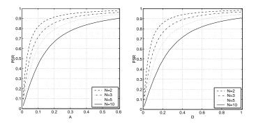
Fig. 5. Energy distribution  $\text{PSR}_{M_{\alpha_j,A}}$  (left) and  $\text{PSR}_{M_{\delta_j,D}}$  (right) of instantaneous DUET estimates around the true mixing parameters. Note, for W-DO signals, the corresponding source energy portion would be 1.0 for all distances from  $\alpha_j$  (and  $\delta_j$ ).
