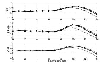
Fig. 4. Window size and type comparison. Hamming ( $\circ$ ), Blackman (\*), Hann ( $\diamond$ ), Triangle ( $\Delta$ ), and Rectangle ( $\Box$ ). PSR, SIR, and WDO for the 0 dB mask for window size = 1, 2, 4, ..., 16384 samples for various window types for pairwise mixing of speech signals sampled at 16 kHz. The Hamming window of size 1024 has the best performance.
