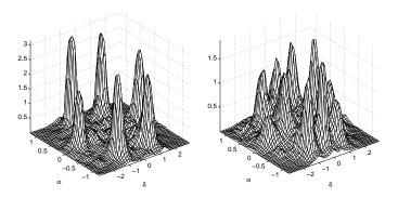
Fig. 8. Six and Ten Source Synthetic Mixing Smoothed Histograms (p = 1). Each peak corresponds to one source and the peak location corresponds to the associated source's mixing parameters.
