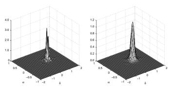
Fig. 7. Example raw (left) and smoothed (right) power weighted (p = 2) histograms for one speech signal in a mixture of five. The peak location of the smoothed histogram corresponds to the mixing parameters ( $\alpha_j, \delta_j$ ) = (0.2, 0.5).
