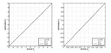
Fig. 14. Histogram Delay (left) and Attenuation (right) Estimator Comparison. The graph on the left compares estimated  $\delta_j$  versus true  $\delta_j$  for the smoothed histogram peak estimators with p = 1/2, 1, 2 for  $\delta_j$  ranging linearly from -5 to 5 samples as  $\alpha_j$  ranges linearly 0.15 to -0.15. The graph on the right compares estimated  $\alpha_j$  to the true  $\alpha_j$ . Both graphs were generated using a model of 5 source mixing.
