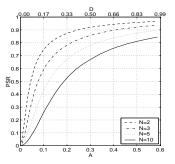
Fig. 6. Energy distribution  $PSR_{M_{\alpha_j}, A}M_{\delta_j, D}$  of instantaneous DUET estimates in a rectangle centered on the true mixing parameter pair  $(\alpha_j, \delta_j)$ .
