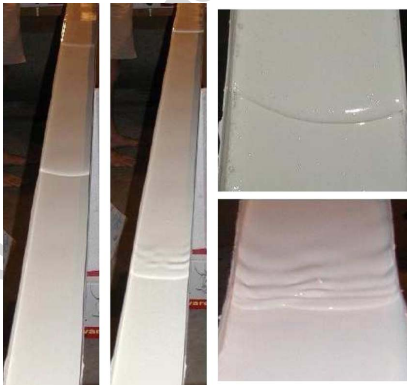
Fig. 23. A kaolin suspension flowing down a channel (width 10 cm, flow depth about 0.5 cm) displays the formation of roll waves. Two experiments are shown; in the first, smooth roll waves appear. In the second, the roll waves develop a secondary instability.
