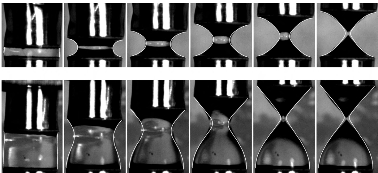
Fig. 19. Experimental and numerical bridge profiles at various times for Carbopol with (top row) \mathcal{W} = 0.99 and L_0 = 0.33 and (bottom row) \mathcal{W} = 0.16 and L_0 = 1.33 . ( N = 100 .)
