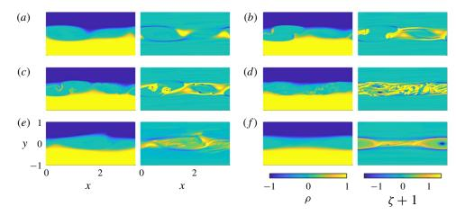
FIGURE 9. (Colour online) Snapshots of the density  $\rho(x, y, t)$  (left) and vorticity  $\zeta(x, y, t) + 1$  (right) for six different times and parameter values in group 5: (*Re*, *Pr*) = (60 000, 3) at (*a*) t = 56, (*b*) t = 66, (*c*) t = 68 and (*d*) t = 86; (*e*) (*Re*, *Pr*) = (20 000, 10) at t = 240, (*f*) (*Re*, *Pr*) = (300 000, 0.6) at t = 250.
