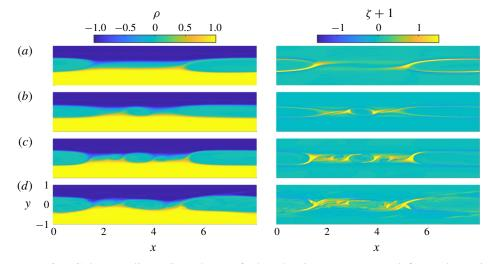
FIGURE 6. (Colour online) Snapshots of the density  $\rho(x, y, t)$  (left) and vorticity  $\zeta(x, y, t) + 1$  (right) for four different times and parameter values in group 1: (a) (Re, Pr) = (300 000, 0.6) at t = 110, (b) (Re, Pr) = (180 000, 1) at t = 141, (c) (Re, Pr) = (20 000, 10) at t = 188 and (d) (Re, Pr) = (20 000, 10) at t = 375. Colour bars show density (left) and vorticity (right).
