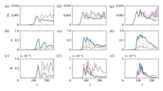
FIGURE 11. (Colour online) Time evolution of (a,d,g) the perturbation energy E(t), (b,e,h) mixing efficiency  $\eta(t)$  and (c,f,i) mixing rate m(t) for the simulations in (a-c) group 2, (d-f) group 3 and (g-i) group 4, with  $(Re, Pr) = (300\,000, 0.6)$  (blue thick solid), (180\,000, 1) (red dashed), (60\,000, 3) (yellow dot-dashed) and (20\,000, 10) (purple thin solid).
