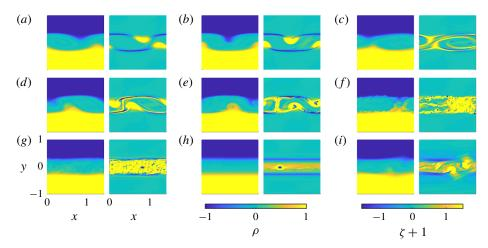
FIGURE 10. (Colour online) Snapshots of the density  $\rho(x, y, t)$  (left) and vorticity  $\zeta(x, y, t) + 1$  (right) for nine different times and parameter values in group 6: (*Re*, *Pr*) = (300 000, 0.6) at (*a*) t = 55, (*b*) t = 62, (*c*) t = 74, (*d*) t = 82, (*e*) t = 88, (*f*) t = 95, (*g*) t = 124 and (*h*) t = 250; (*i*) (*Re*, *Pr*) = (20 000, 10) at t = 200.
