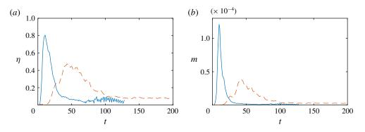
FIGURE 4. (Colour online) (a) Instantaneous mixing efficiency  $\eta(t)$  and (b) instantaneous mixing rate m(t) for representative KHI (blue solid) and HWI (red dashed, for which we plot 10m(t)) simulations.
