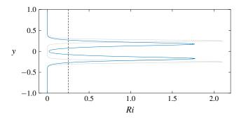
FIGURE 7. (Colour online) Gradient Richardson number  $-J\rho_y/u_y^2$  for the horizontally averaged buoyancy and velocity profiles in the region between the billow 2.4 < x < 4.2 for the (*Re*, *Pr*) = (300 000, 0.6) group 1 simulation at t = 110 (blue), along with the gradient Richardson number for the initial condition (grey, dotted). Also shown is the value Ri = 0.25 (black dashed).
