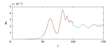
FIGURE 14. (Colour online) Evolution of the perturbation kinetic energy for the 2-D simulation with (Re, Pr) = (20000, 10) in group 6 (thin blue) and a 3-D simulation initialised by randomly perturbing the 2-D simulation at t = 50 (thick red).
