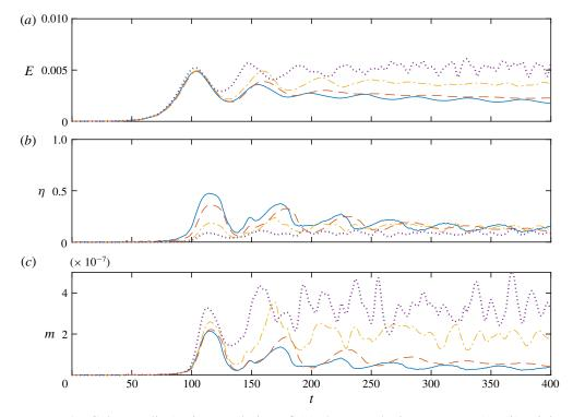
FIGURE 5. (Colour online) Time evolution of (a) the perturbation energy E(t), (b) mixing efficiency  $\eta(t)$  and (c) mixing rate m(t) for the simulations in group 1, with (*Re*, *Pr*) = (300 000, 0.6) (blue solid), (180 000, 1) (red dashed), (60 000, 3) (yellow dot-dashed) and (20 000, 10) (purple dotted).
