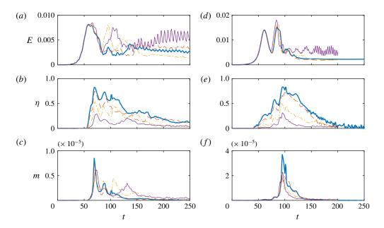
FIGURE 8. (Colour online) Time evolution of (a,d) the perturbation energy E(t), (b,e) mixing efficiency  $\eta(t)$  and (c,f) mixing rate m(t) for the simulations in (a-c) group 5 and (d-f) group 6, with  $(Re, Pr) = (300\,000, 0.6)$  (blue thick solid),  $(180\,000, 1)$  (red dashed),  $(60\,000, 3)$  (yellow dot-dashed) and  $(20\,000, 10)$  (purple thin solid).
