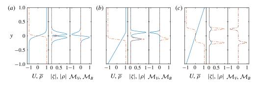
FIGURE 1. (Colour online) Columns from left to right: sample background profiles U(y) (blue solid) and  $\bar{\rho}(y)$  (red dot-dashed) for (a) KHI, (b) HWI and (c) TCI. Absolute value of vorticity (blue) and density (red dot-dashed) for the associated growing mode.  $\mathcal{M}_V$  (blue solid, when non-zero) and  $\mathcal{M}_B$  (red dot-dashed) for the background profiles and the associated modes.
