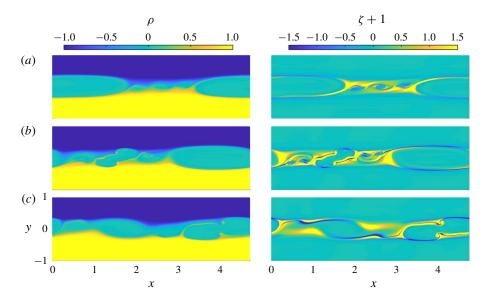
FIGURE 12. (Colour online) Snapshots of the density  $\rho(x, y, t)$  (left) and vorticity  $\zeta(x, y, t) + 1$  (right) for three different times and parameter values in groups 2, 3 and 4: (*Re*, *Pr*) = (20000, 10) for (*a*) J = 0.14 at t = 169, (*b*) J = 0.23 at t = 104 and (*c*) J = 0.3 at t = 93.
