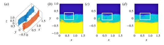
FIGURE 15. (Colour online) (a) Surfaces of  $\rho = -1/2$  (blue) and  $\rho = 1/2$  (red) at t = 100 for a (*Re*, *Pr*) = (20000, 10) 3-D simulation simulation of group 6. (b) Vertical slice through the 3-D density field at t = 100, and (*c*,*d*) the 2-D density fields at t = 100 and 102. White boxes highlight a feature detaching from the upper density interface. Density colour bar as in figures 6, 9, 10 and 12.
