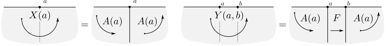
Fig. 7. In Fig. 6 the eigenvectors X and Y were recast as matrices. Now we rewrite them again as products of the matrix F together with the corner transfer matrix A . The matrix F sweeps through a half-row or half-column and the matrix A sweeps through a quarter of the lattice.
