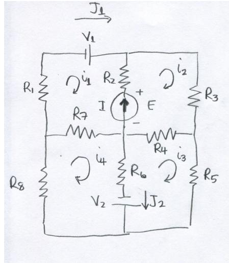
**A20:** Consider the resistor network above. Using the loop current method you have learned in the lectures and labs, write the equation for voltages around loop 1. Your equation should have the resistances and sources as parameters.
